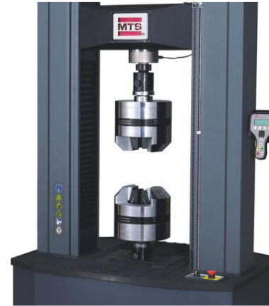
Universal Testing Machine (UTM) Dynamic 100 kN
