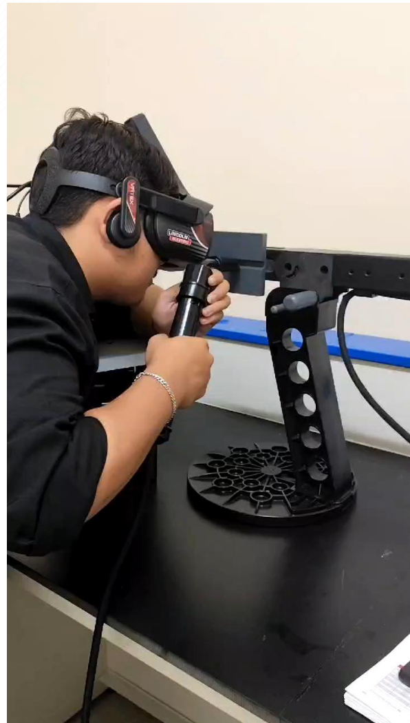
Simulated Welding Training Machine (dual user)
